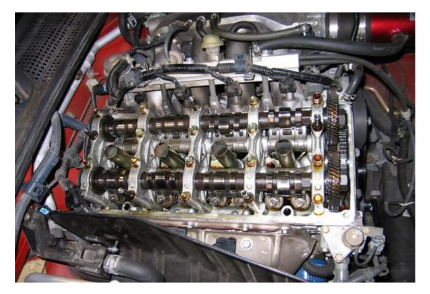
2) Make sure the car is in neutral. Use the 19mm wrench on the crankshaft bolt to turn the engine to TDC for cylinder #1: the marks on the cam gears will align as shown below (page 6-12 in the Helm manual).
