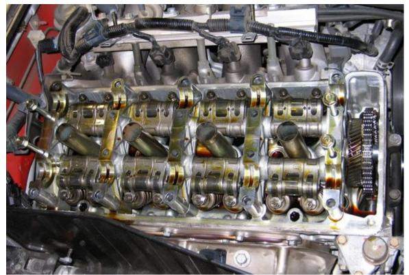
d) If you're just replacing retainers, it's not necessary to remove the rocker arm assembly. Just rotate the rockers/followers up off of the springs, exposing the retainers.
